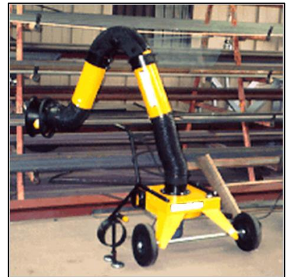
Local Exhaust Ventilation
